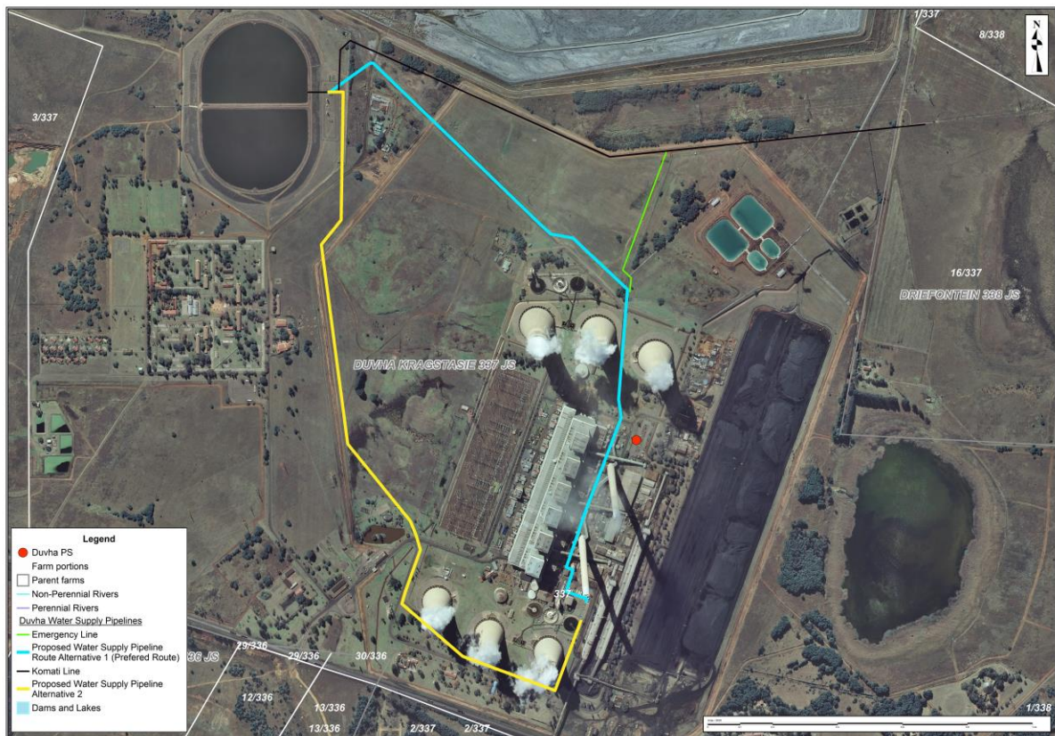
Figure 1: Location of the proposed water supply pipeline
